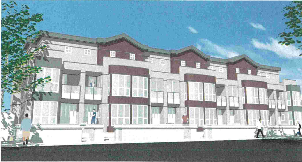
Figure 3.30 Burnt Sienna colour scheme with charcoal accents. New cross-cavity flashing and metal cap flashings are installed with a charcoal colour. Balcony guardrails match the colour of metal flashings and incorporate full height guardrails with privacy glass and clear glass panel guardrails.
