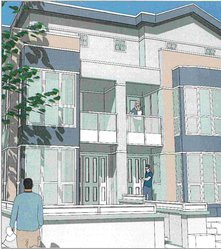
Figure 3.12 A guardrail scheme with a mix of clear and opaque glass panels that extend to the underside of the balcony edge could enhance the appearance of the building.
