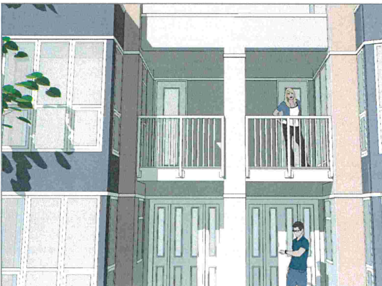
Figure 3.9 An approach of omitting the guard walls and replacing them with new face- mounted guardrails should be considered.
