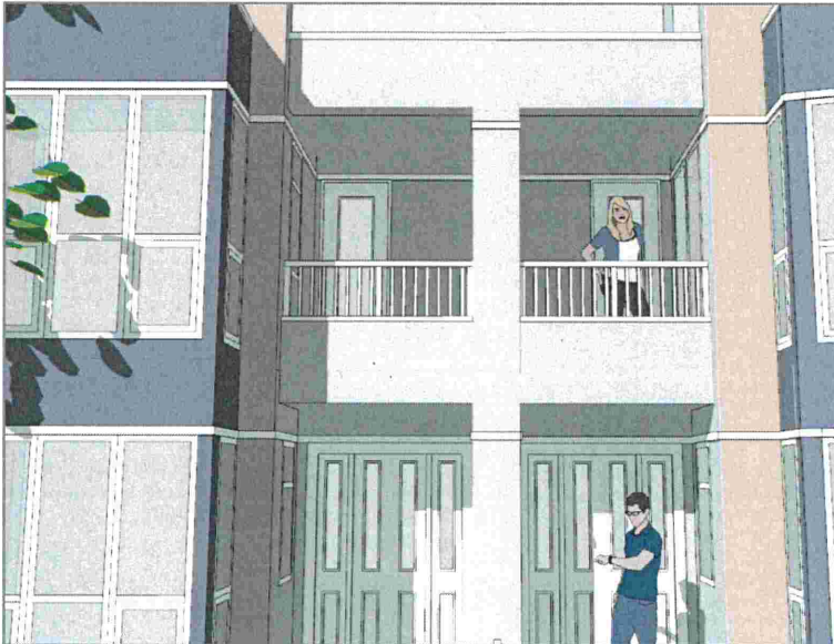
Figure 3.8 The existing condition with a combination of guardrails and stucco clad guard walls could be reproduced during rehabilitation; however, there are benefits to other approaches.
