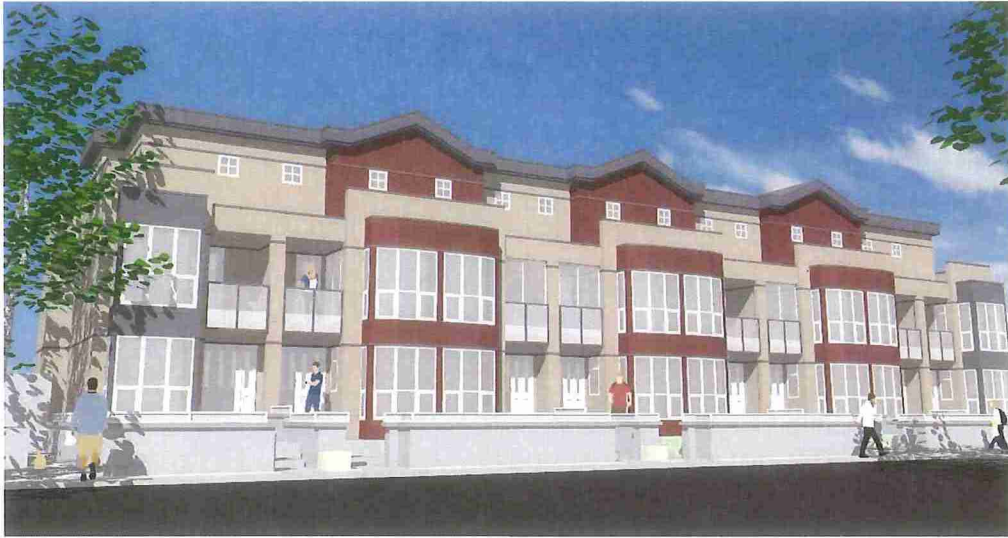
Figure 3.30 Burnt Sienna colour scheme with charcoal accents. New cross-cavity flashing and metal cap flashings are installed with a charcoal colour. Balcony guardrails match the colour of metal flashings and incorporate full height guardrails with privacy glass and clear glass panel guardrails.
